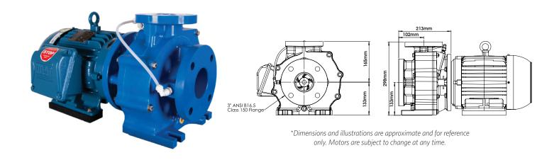
The GENESYS® 3x2-6 vinyl ester and polyester end-suction centrifugal pump line is designed and engineered to provide highly efficient pumping solutions. The fiberglass reinforced polymer case construction with the option of no wetted metal parts gives it compatibility with many aggressive chemistries and corrosive fluids. The unique enclosed-impeller and time-tested volute design render 2 pole BEP performance at 78% efficiency.
