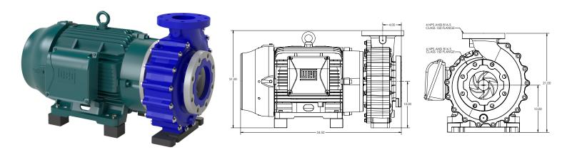
The GENESYS® 6x4-11 vinyl ester and polyester end-suction centrifugal pump line is designed and engineered to provide highly efficient pumping solutions. The fiberglass reinforced polymer case construction with the option of no wetted metal parts gives it compatibility with many aggressive chemistries and corrosive fluids. The unique enclosed-impeller and time-tested volute design render 1800 RPM performances at 79% efficiency.
